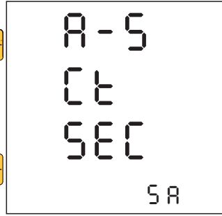
Current setting of CT secondary side 1A/5A/333mV (If default is 333mV, it cannot be changed)
