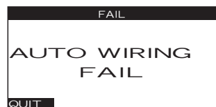
Wiring change failure Press Enter to QUIT
