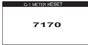
G-1 Meter reset After inputting 7170, it will reboot and return to default value, but the adjusted value will be retained.
